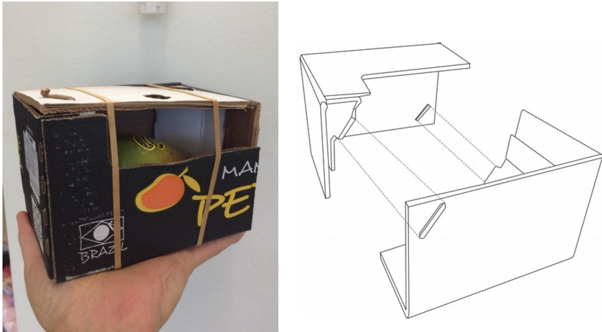
Figure 3: Design of a "Mango Equivalent Unit" (MEU)
